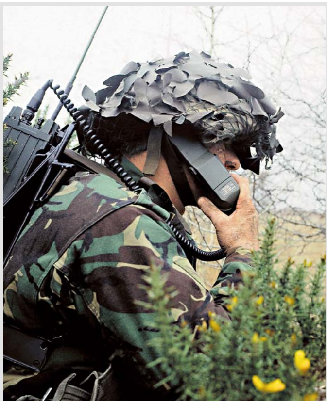
Significant among recent changes is the need to provide control functions on the handset in addition to the radio front panel.
